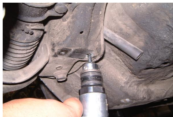
Drill out slotted mounting holes (Fig. 2)
