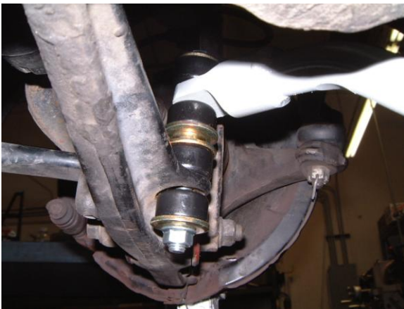
Passenger side end link assembly (Fig. 5)
