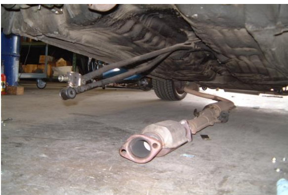
Drop the exhaust and shifter linkage (Fig. 1)
