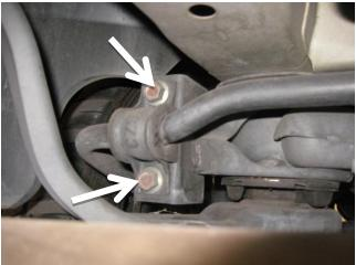
6. Locate the pivot "D" shaped polyurethane bushing and tube of special grease supplied in the hardware kit. Cut the end off the tube and apply grease to the bore of the bushing. Open bushing and snap them over the new sway bar, as positioned on the stock bar.
