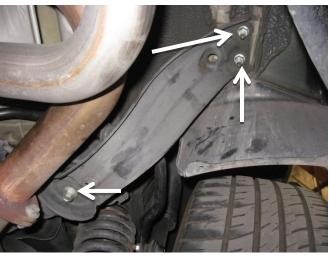
5. Use a 6mmm allen wrench to hold the end link stud and a box wrench to loosen the nut. Separate the end links from the sway bar. Remove the factory bushings and brackets. The fasteners will be reused for installation. Remove the sway bar from the vehicle.
