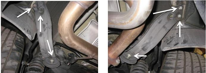
9. Connect and tighten the exhaust, careful not to damage the gasket.
