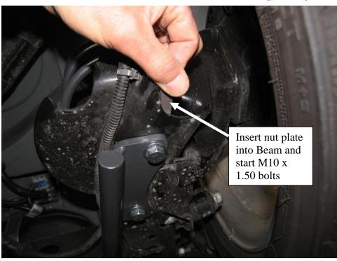
Insert Nut plate into end of beam and thread bolts into the nuts.
