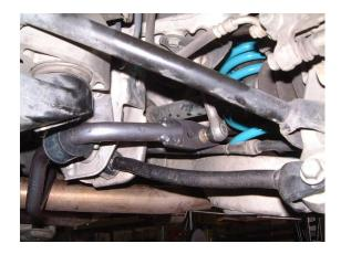
**4.** Locate the pivot "D shaped" polyurethane bushings and tube of special grease supplied in the hardware kit. Cut the end off the grease tube and apply the grease to the bore of the polyurethane bushings (in the hole). Open the bushings and snap them over the new anti-sway bar, as positioned on the stock bar. Place the new brackets (supplied) over the pivot bushings. Tighten brackets using factory hardware to OEM specifications.
